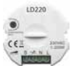
FD-LD220 Dimmer for LED lamp Power: 200W 230V 50/60 Hz Installed in the mounting box behind the push button. Dimensions: 56 x 22 mm Units: 1
